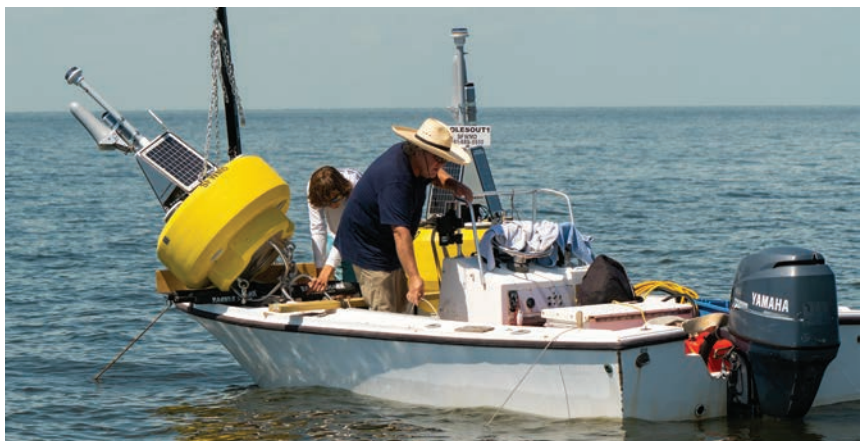
SFWMD Staff Deploying Nexsens CB 450 Data Buoys on Lake Okeechobee to Help Monitor Water Quality Across the Lake. (Photo by SFWMD)
